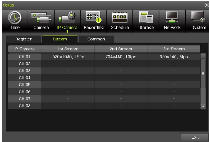
[Figure 3-19. IP Camera Stream Setup]
