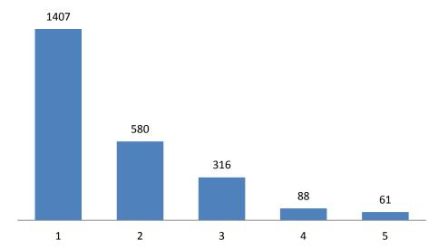
From a total of 2452 pipe segments inspected, 1407 segments were found to be in acceptable structural condition (Grade 1), 580 segments were found to be in minimal collapse risk condition (Grade 2), 316 segments were in collapse unlikely in near future condition (Grade 3), 88 segments were found to be in collapse likely in foreseeable future condition (Grade 4); and 61 segments were found to be in danger of imminent collapse (Grade 5).
