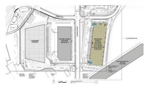
Figure 2. Site plan for Phase 2 showing container storage area and 2 new buildings.
