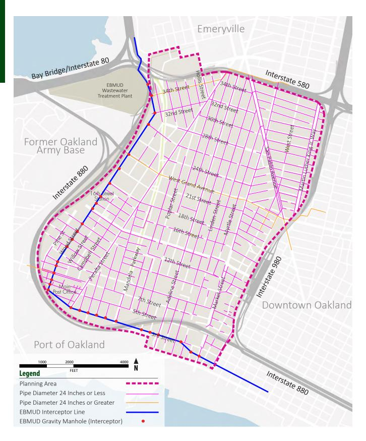
Most of the City's sewer system is over 50 years old, some as old as 100 years. Most of the sewer pipes are in poor condition, and many are plugged or abandoned. Much of the City's antiquated sewer system is constructed of vitrified clay pipe, making it susceptible to cracking and vulnerable to failure. Many pipes do not have any associated data, such as diameter, flow direction, material, etc.
