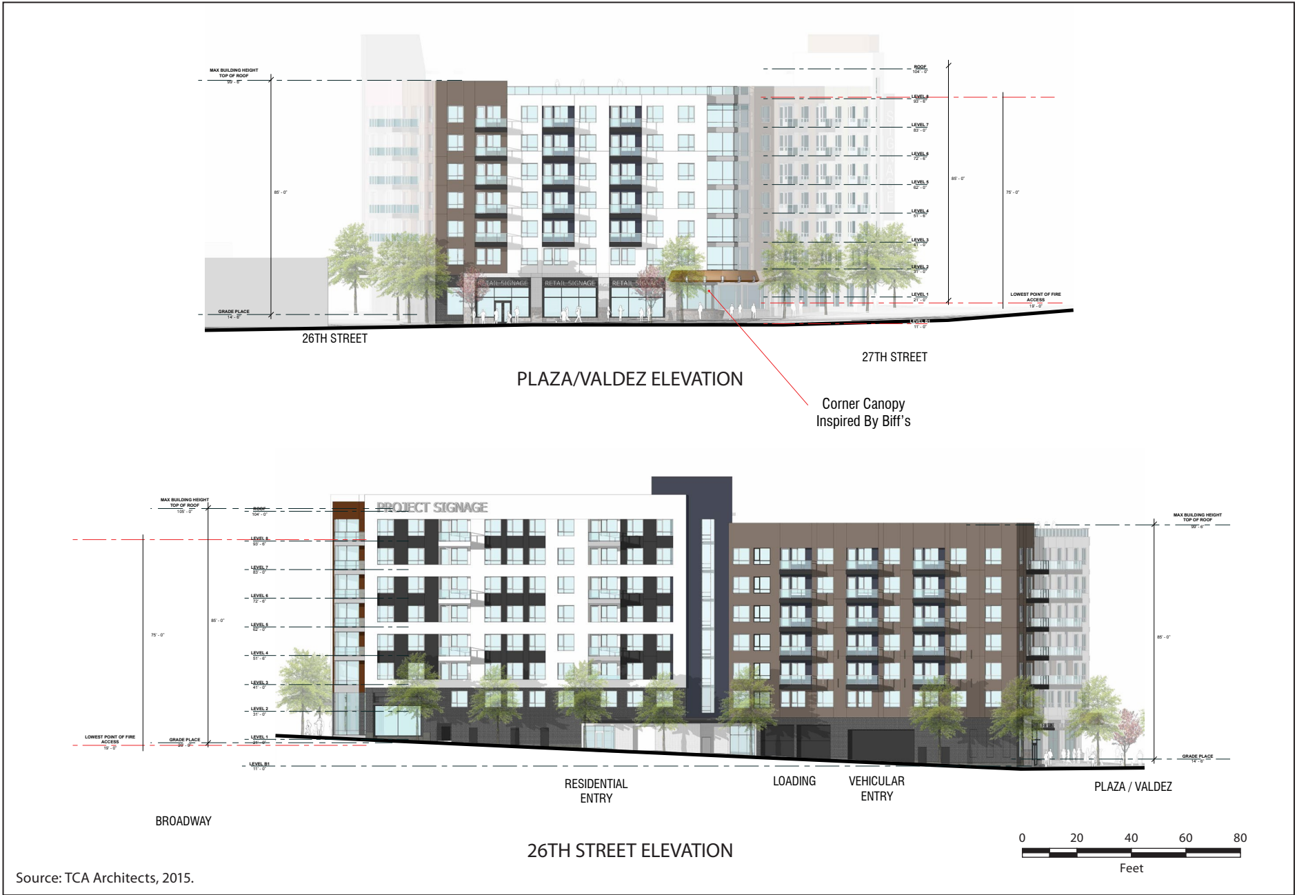
Figure 3 Massing Elevations – Plaza and 26th Street Broadway and 27th Project
