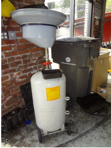
Photo 7: Representative view of used oil drainage tanks.
