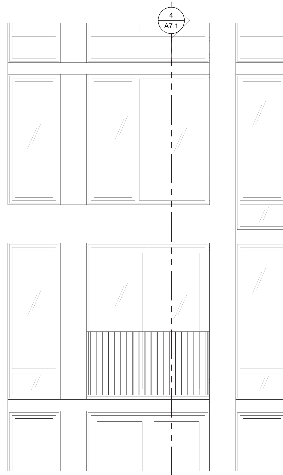
5 MID-RISE ELEVATION DETAIL SCALE: 3/8" = 1'-0"
