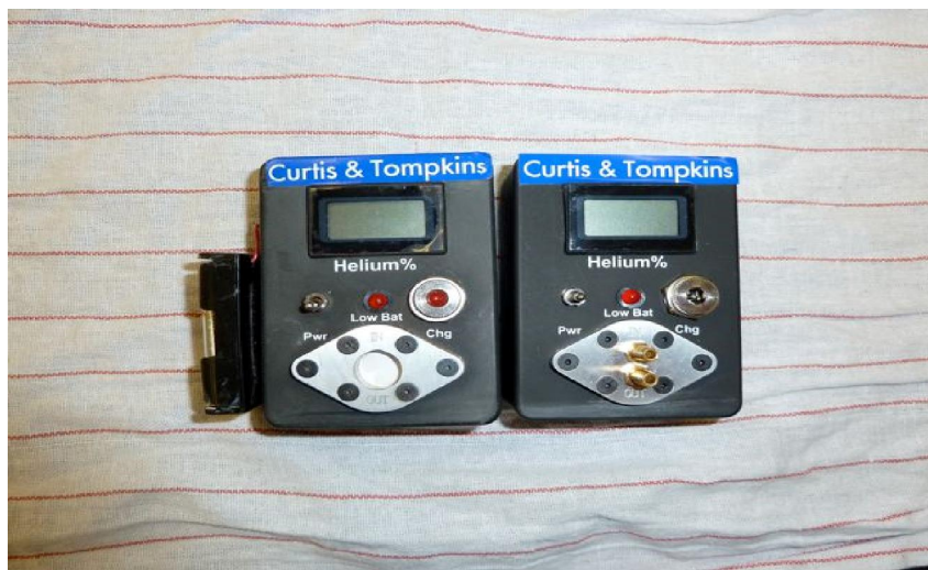
Figure 1: Diffusion Cell (left) and Flow-Through cell (right) Helium Detectors
