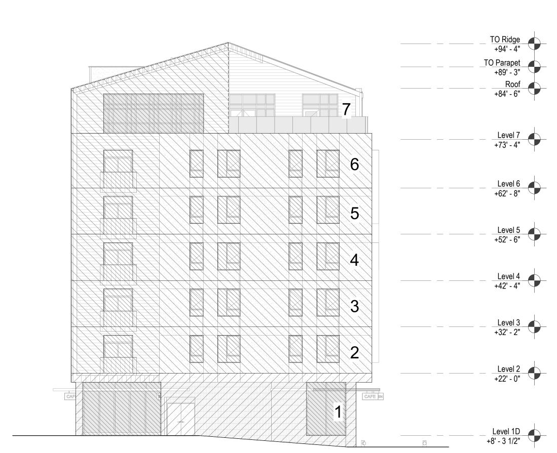
BUILDING ELEVATION - WEST (OPENING PROTECTION)
