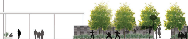
Metal "Bamboo" Screen Elevation The screen provides a separation between passive and active activity areas and protects passive users from basketballs.
