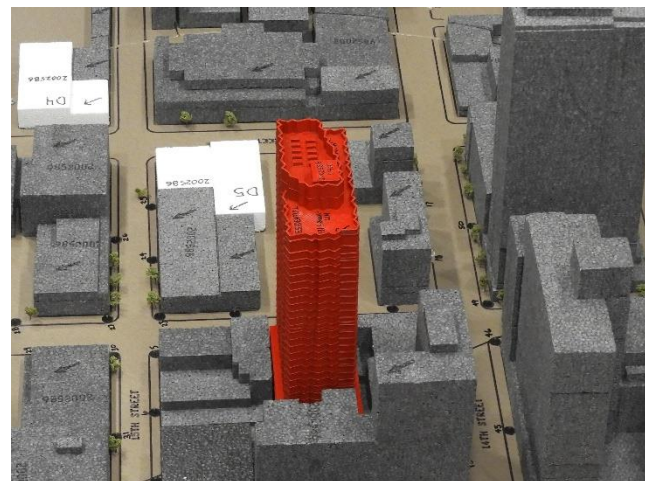
Image 2C: Wind Tunnel Study Model – Existing + Project (Residential) Configuration
