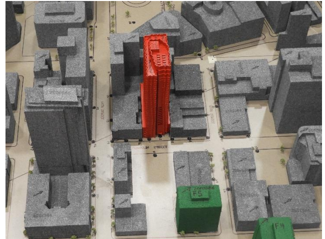
Image 2E: Wind Tunnel Study Model – Project (Residential) + Cumulative Configuration
