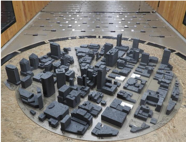
Image 2A: Wind Tunnel Study Model – Existing Configuration
