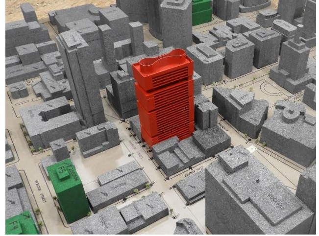
Image 2D: Wind Tunnel Study Model – Project (Office) + Cumulative Configuration
