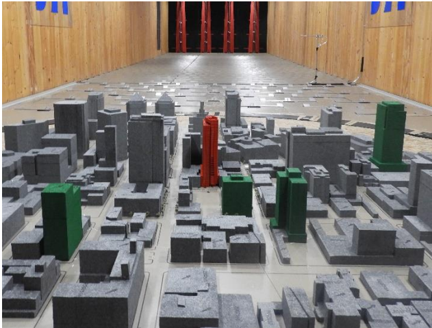
Image 2E: Wind Tunnel Study Model – Project (Residential) + Cumulative Configuration
