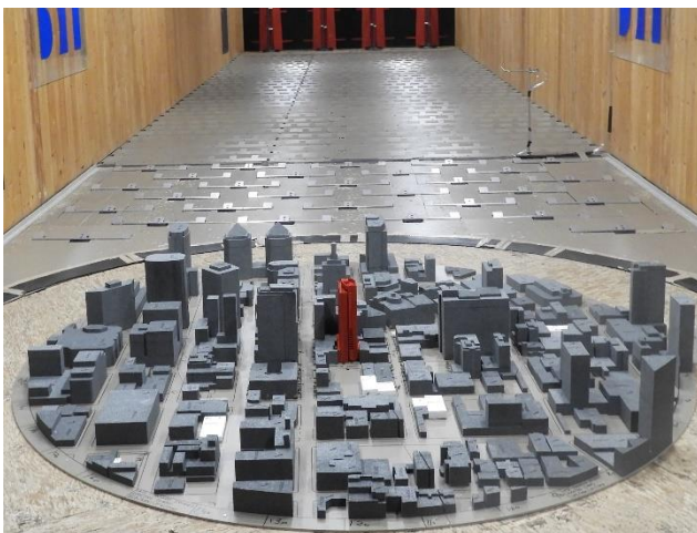
Image 2C: Wind Tunnel Study Model – Existing + Project (Residential) Configuration
