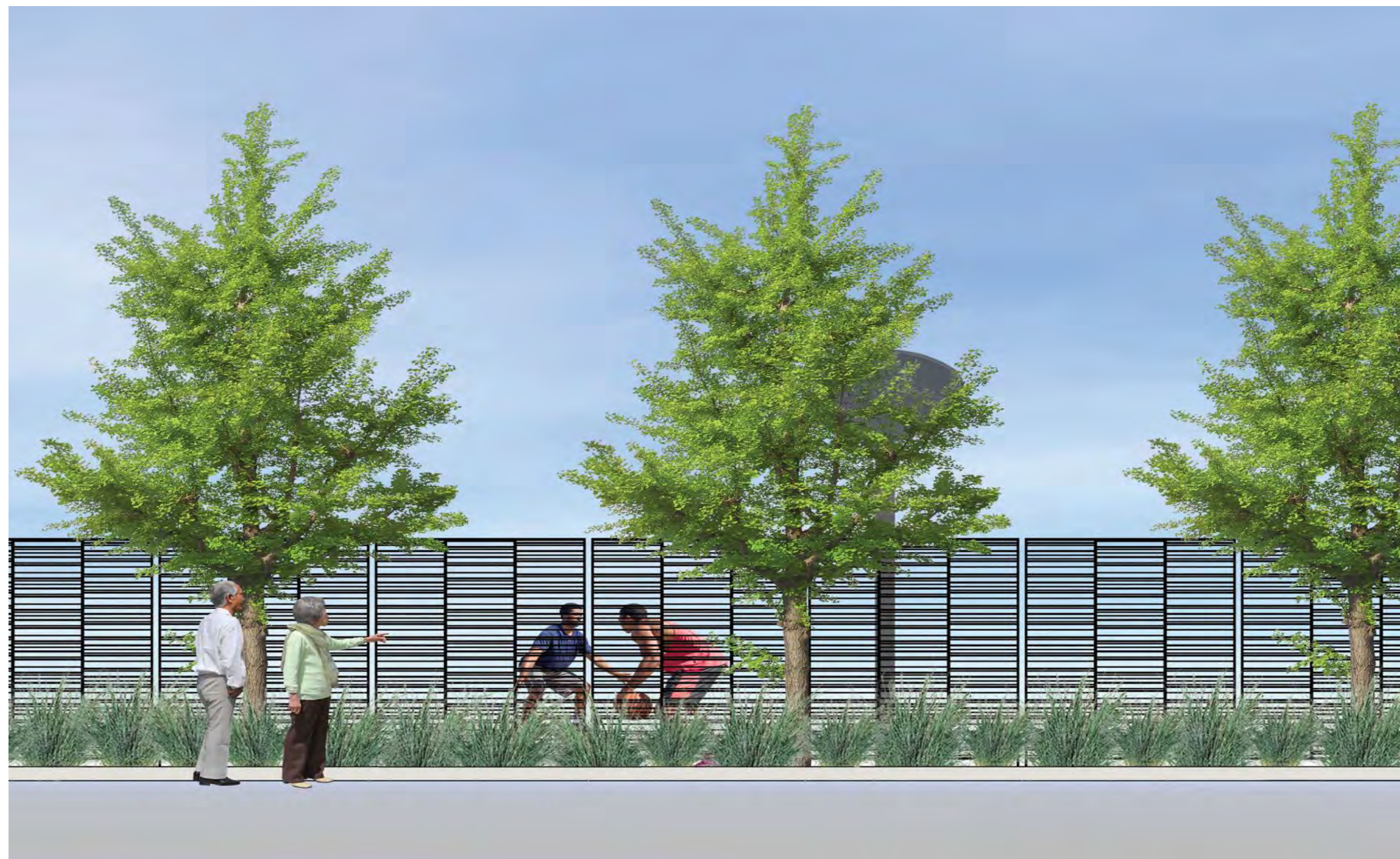
PLAZA PROTECTION SCREEN RENDERING SHOWING ACTUAL DESIGN AND TRANSPARENCY BLACK STEEL CONSTRUCTION
