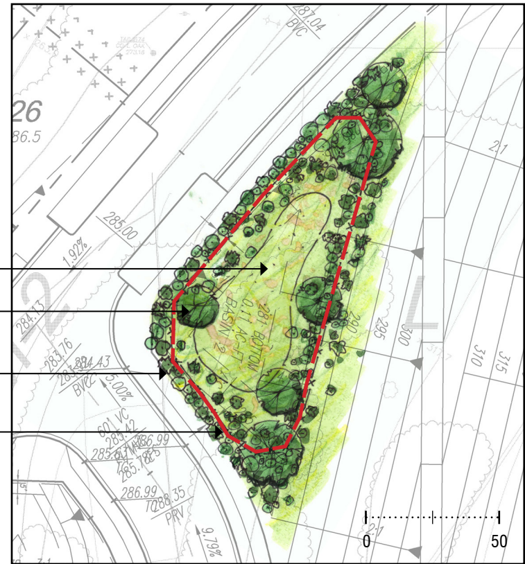
Figure 29 - Typical Detention Basin Plan
