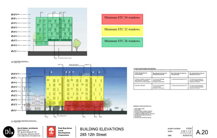
Figure 9 Recommendations for Noise Insulation –
