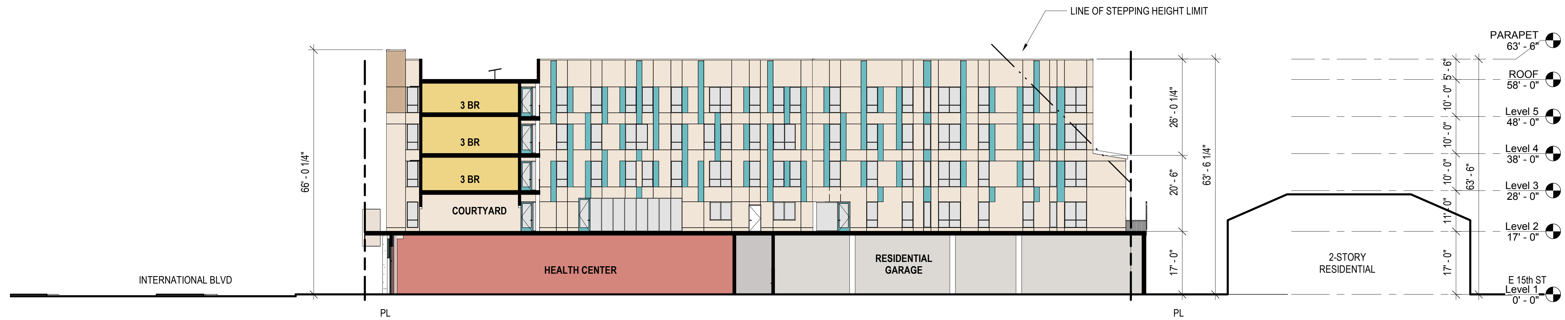
NORTH-SOUTH SECTION THROUGH WEST WING ① 1/16" = 1'-0"
