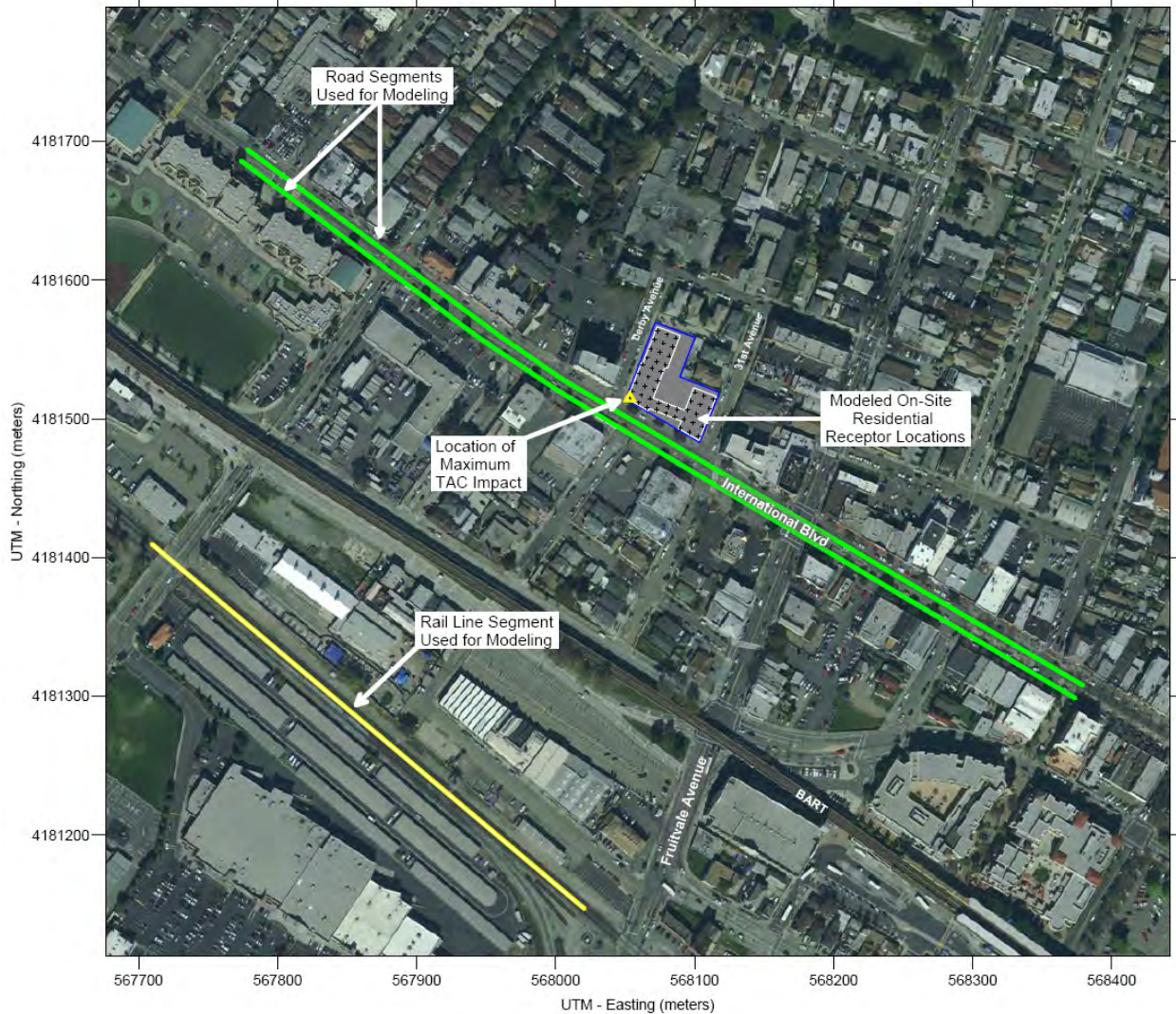
Figure 2. Project Site, On-Site Sensitive Receptors, Roadway and Rail Line Segments Modeled, and Receptor with Maximum TAC Impacts
