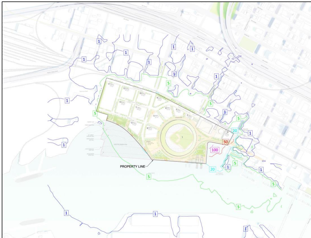
Figure 292: Spill light map for MRA project, Baseline ballpark height, "Full Buildout" scenario Game Night lighting condition indicating vertical illuminance isolines
