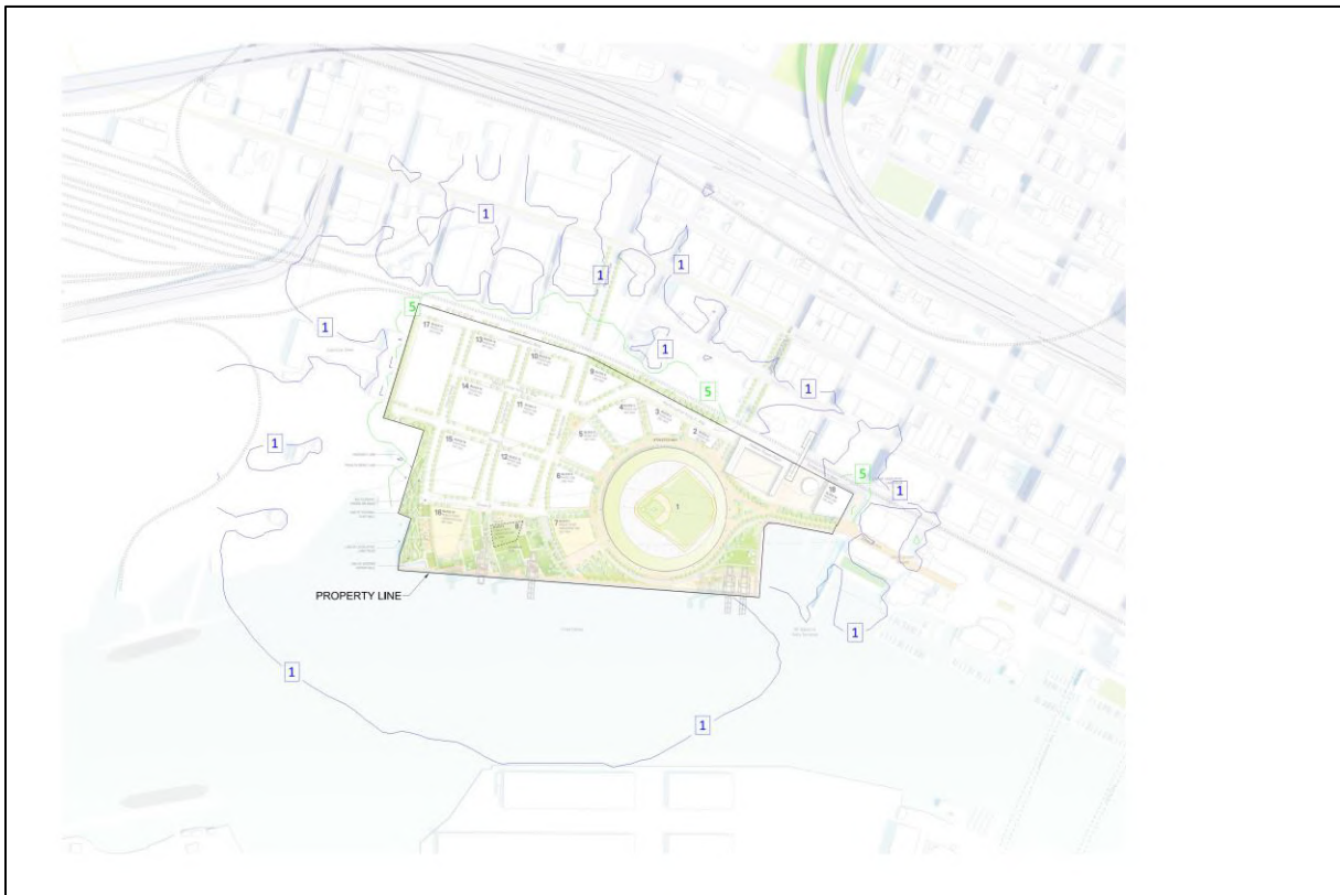
Figure 170: Spill light map for Baseline project, Baseline ballpark height, "Full Buildout" scenario Post-Curfew lighting condition indicating vertical illuminance isolines
