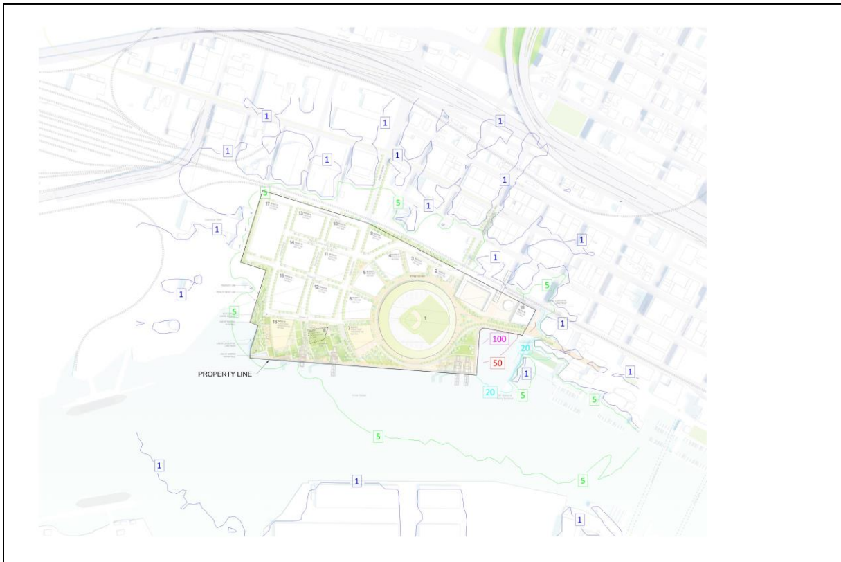
Figure 199: Spill light map for Baseline project, Reduced ballpark height, "Full Buildout" scenario Game Night lighting condition indicating vertical illuminance isolines
