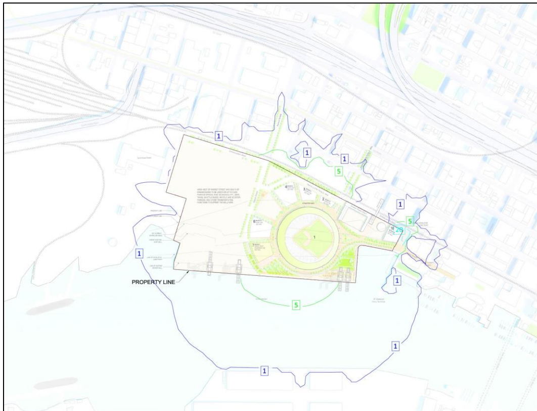
Figure 102: Spill light map for Baseline project, Baseline ballpark height, "Phase 1" scenario Non-Game Night, Pre-Curfew lighting condition indicating vertical illuminance isolines
