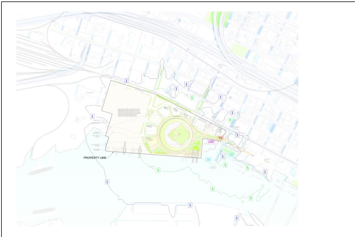
Figure 85: Spill light map for Baseline project, Baseline ballpark height, "Phase 1" scenario Game Night lighting condition indicating vertical illuminance isolines
