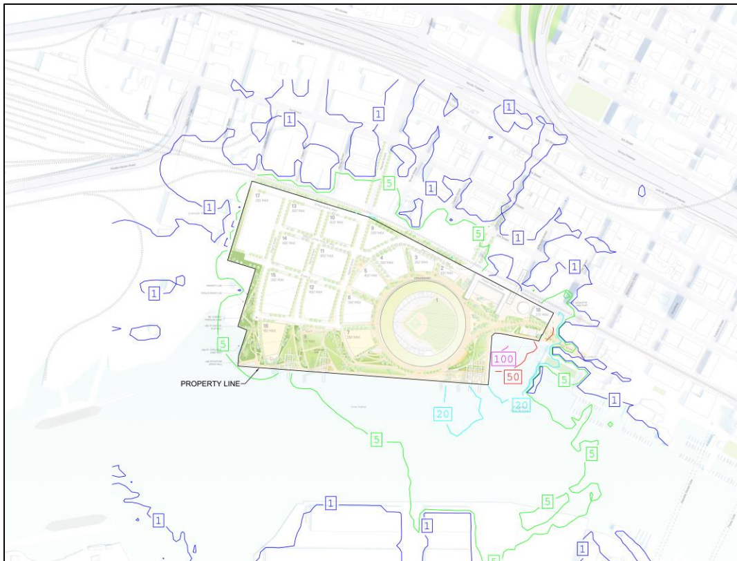
Figure 223: Spill light map for Baseline project, Rotated Ballpark design option, "Full Buildout" scenario Game Night lighting condition indicating vertical illuminance isolines
