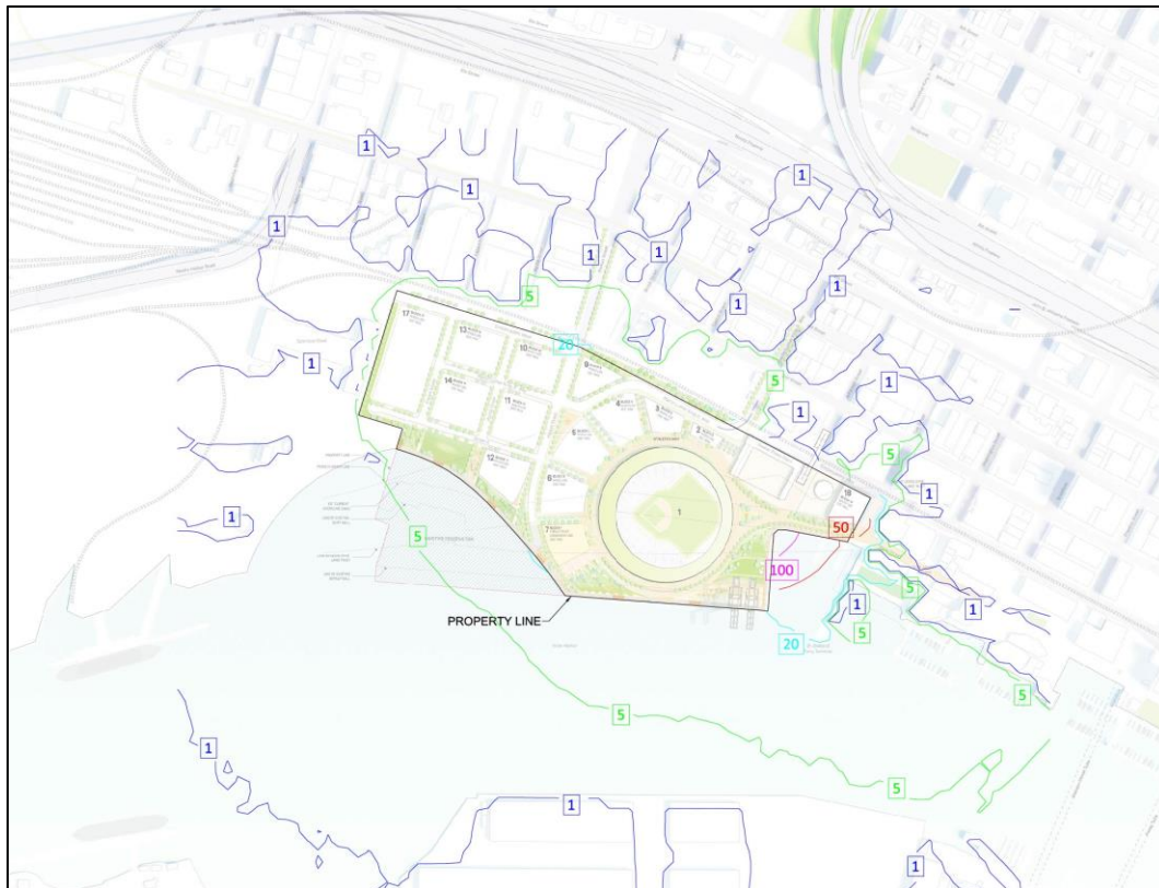
Figure 355: Spill light map for MRA project, Reduced ballpark height, "Full Buildout" scenario Game Night lighting condition indicating vertical illuminance isolines
