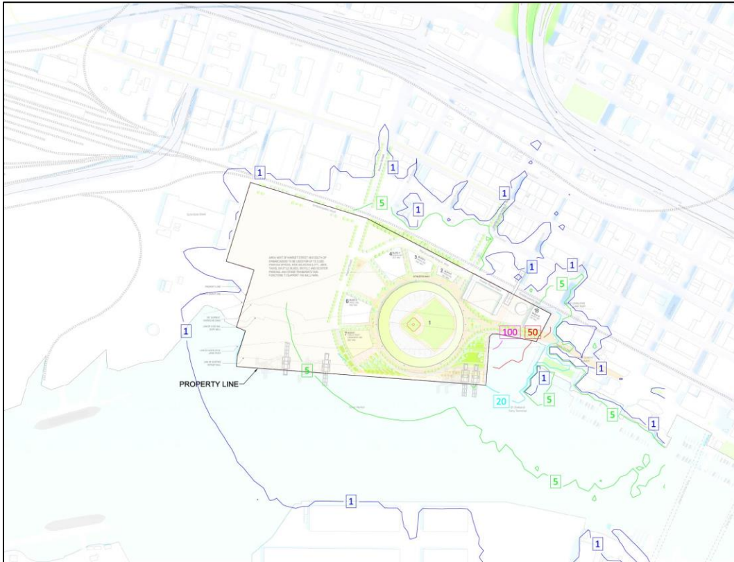
Figure 241: Spill light map for MRA project, Baseline ballpark height, "Phase 1" scenario Game Night lighting condition indicating vertical illuminance isolines
