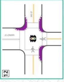
Based on truck turning requirements, provide curb extensions on 3rd Street at Market Street to shorten the Market Street crossing distance and on the north side of Market Street to shorten the crossing distance on the north side of the intersection.
