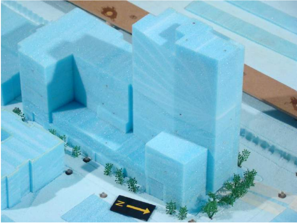
Figure 2. Photographs of the completed model in the wind tunnel: (i) Close-up view of proposed structure with Landscape Option 2.
