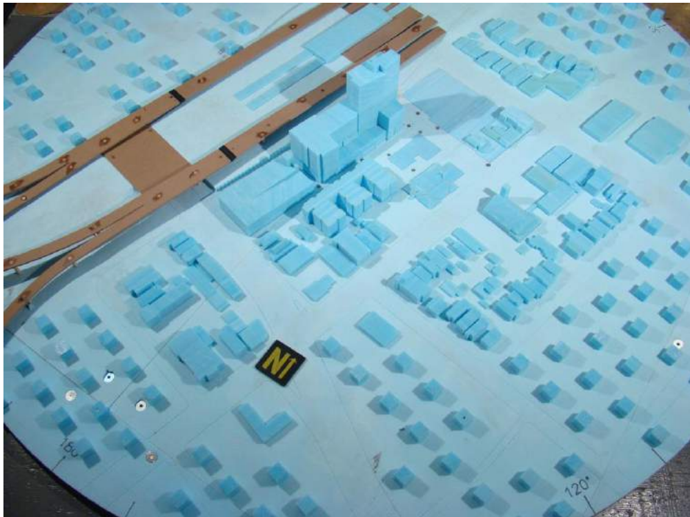
Figure 2. Photographs of the completed model. Overhead views of the completed model in the wind tunnel: (c) Configuration A (Existing); (d) Configuration B (Existing-plus-Proposed).
