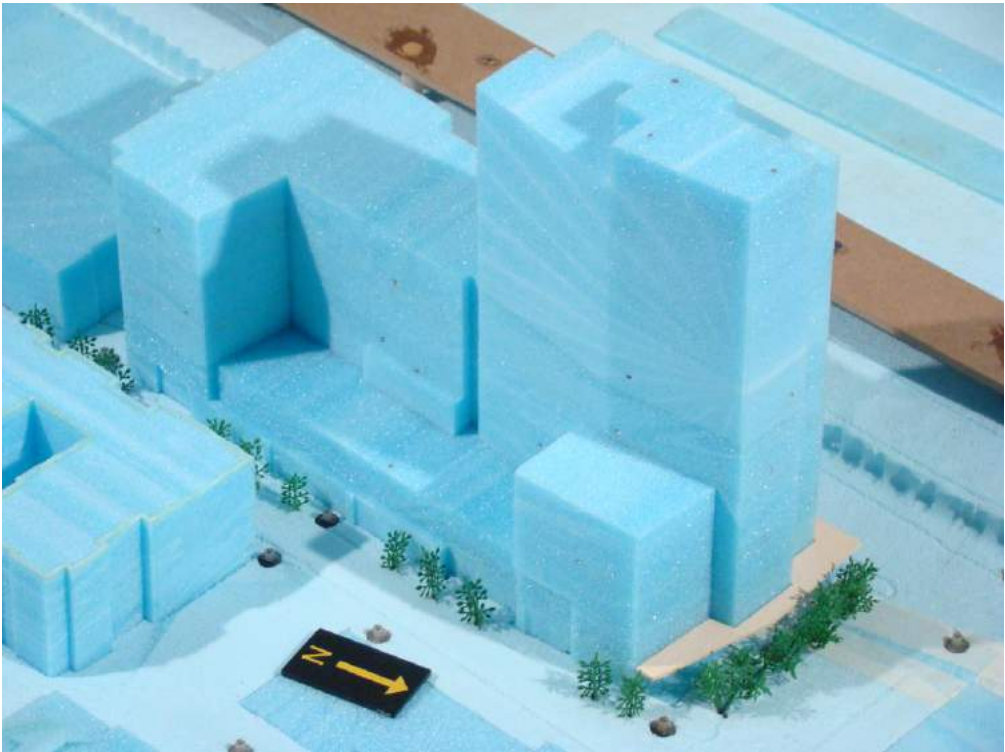
Figure 2. Photographs of the completed model in the wind tunnel: (g) Close-up view of proposed structure; (h) Close-up view of proposed structure with Landscape Option 1 + Canopy.
