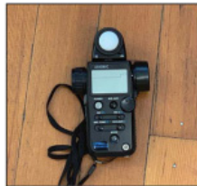
Figure 27: Light meter used for luminance and illuminance measurements
