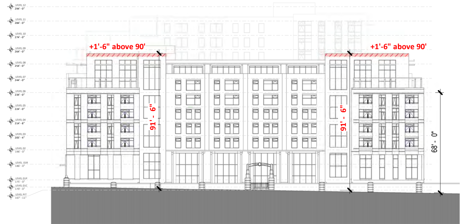
ELEVATION - BUILDING A WEST 1" = 40'-0"
