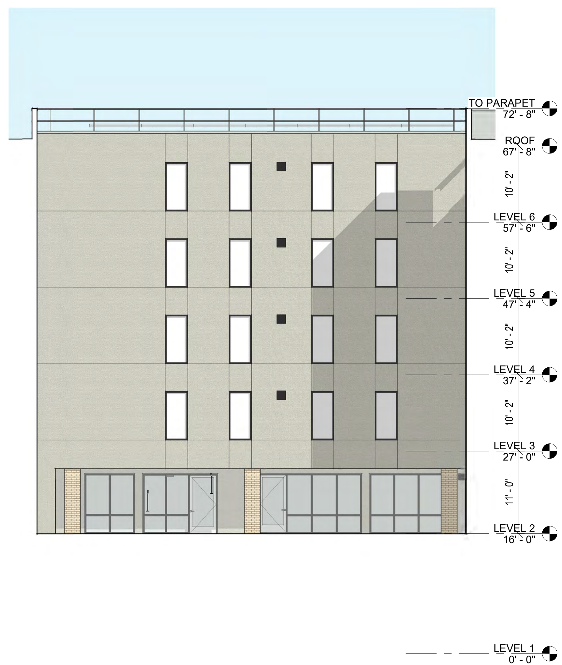
SOUTH COLOR ELEVATION - COURTYARD ③ 1/8" = 1'-0"
