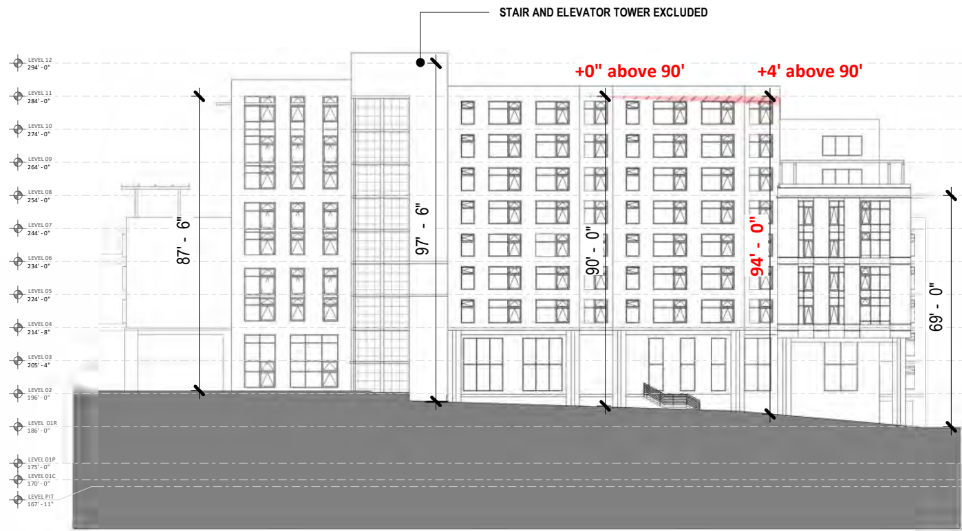
ELEVATION - BUILDING A EAST 1" = 40'-0"
