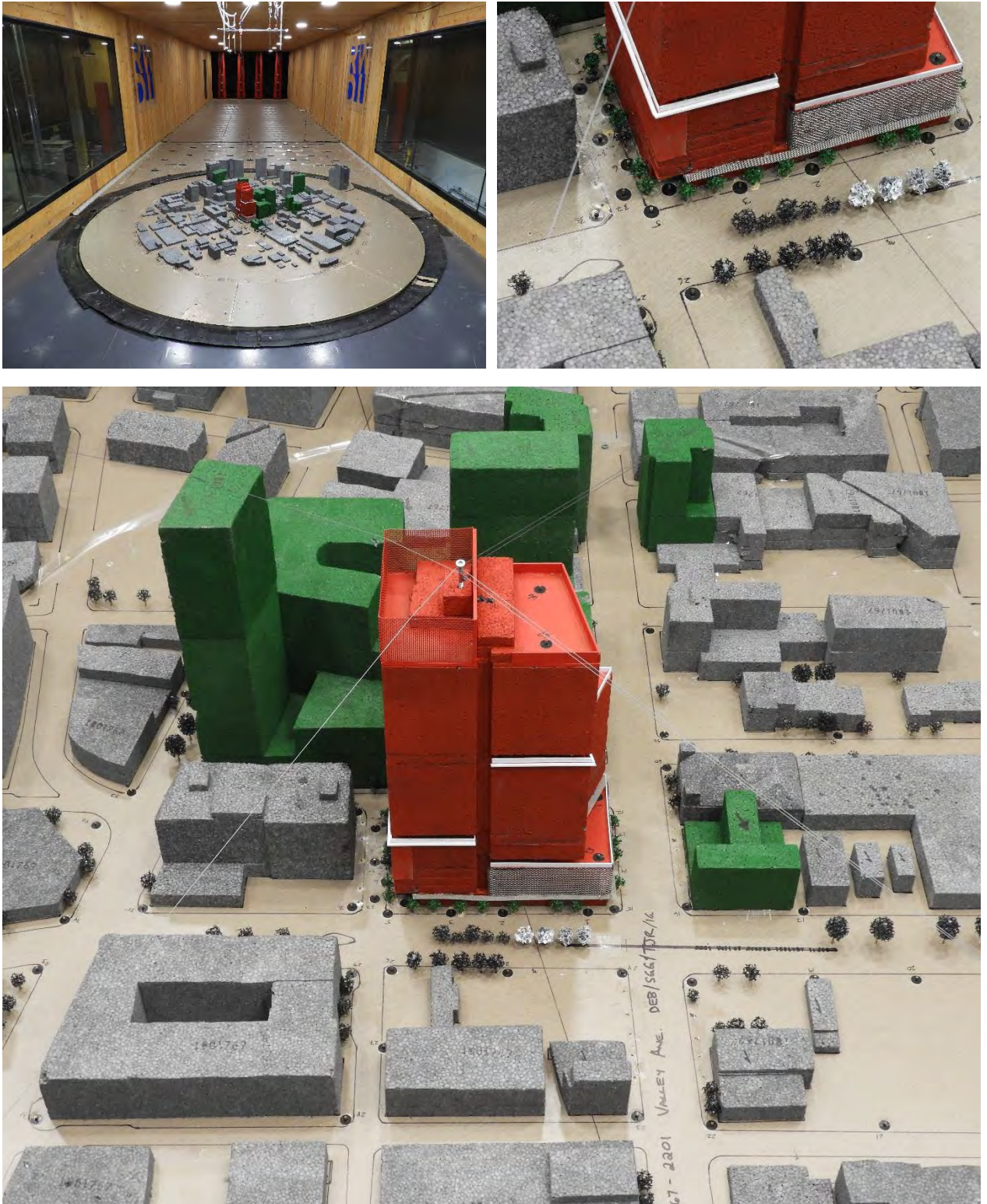
Image 2e: Wind tunnel study model – Project + Cumulative + Median Trees configuration
