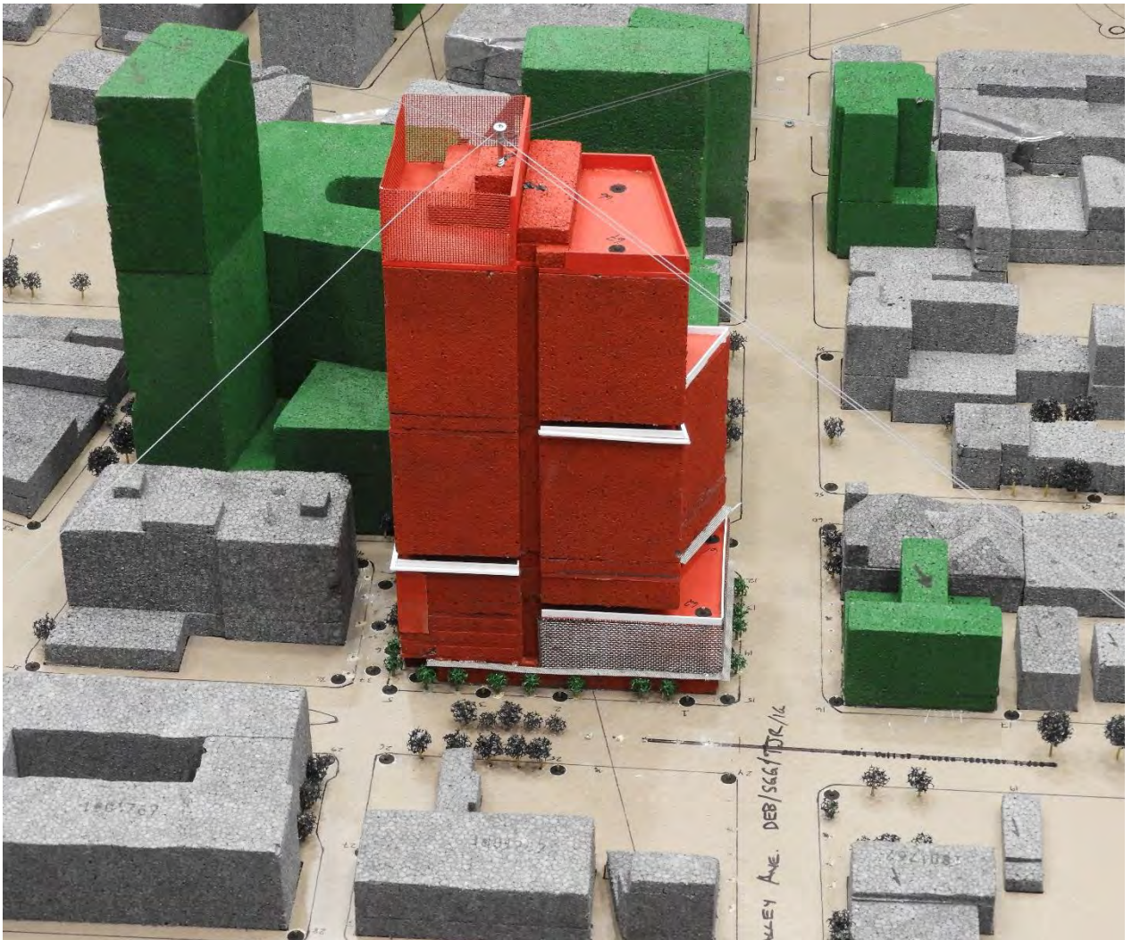
Image 2d: Wind tunnel study model – Project + Cumulative configuration
