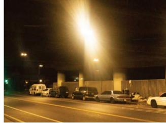
Example of glare caused by existing luminaires
