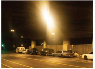
Example of glare caused by existing luminaires
