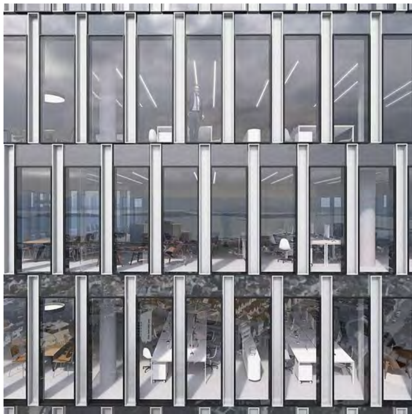
CURTAIN WALL HIGH SOLAR PERFORMANCE WINDOW SYSTEM
