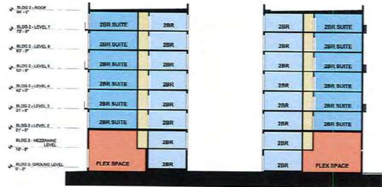
1) BUILDING 2 - SECTION THROUGH COURT 1/16" = 1'-0"
