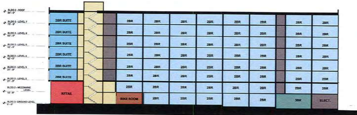
3) BUILDING 2 - SECTION THROUGH UNITS 1/16" = 1'-0"
