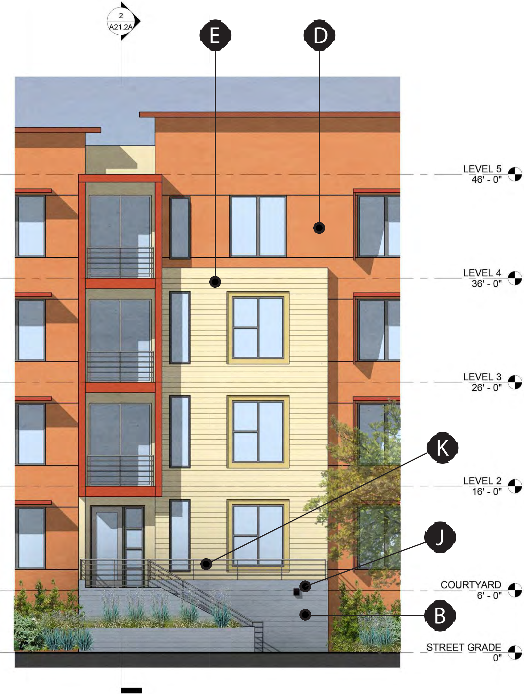
1 NORTH ELEVATION - TYPICAL STOOP 3/16" = 1'-0"
