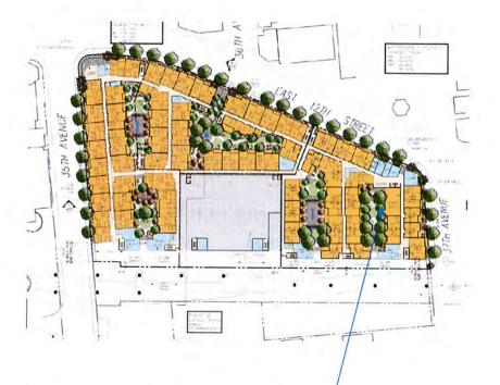
**Revised 2015 FPUD Site Plan for Phase IIA that affect Phase IIB shows** changes in the parking garage affecting both properties. The location of the parking is still along the BART tracks but it is incorporated into the 4-story housing development. Open space is moved to the interior and the future shared 'Paseo' between Phase IIA and Phase IIB is identified. This is an enlargement of half of the original PUD site plan
