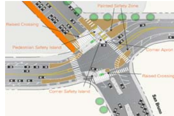
9 th /Division protected intersection (I-80), San Francisco
