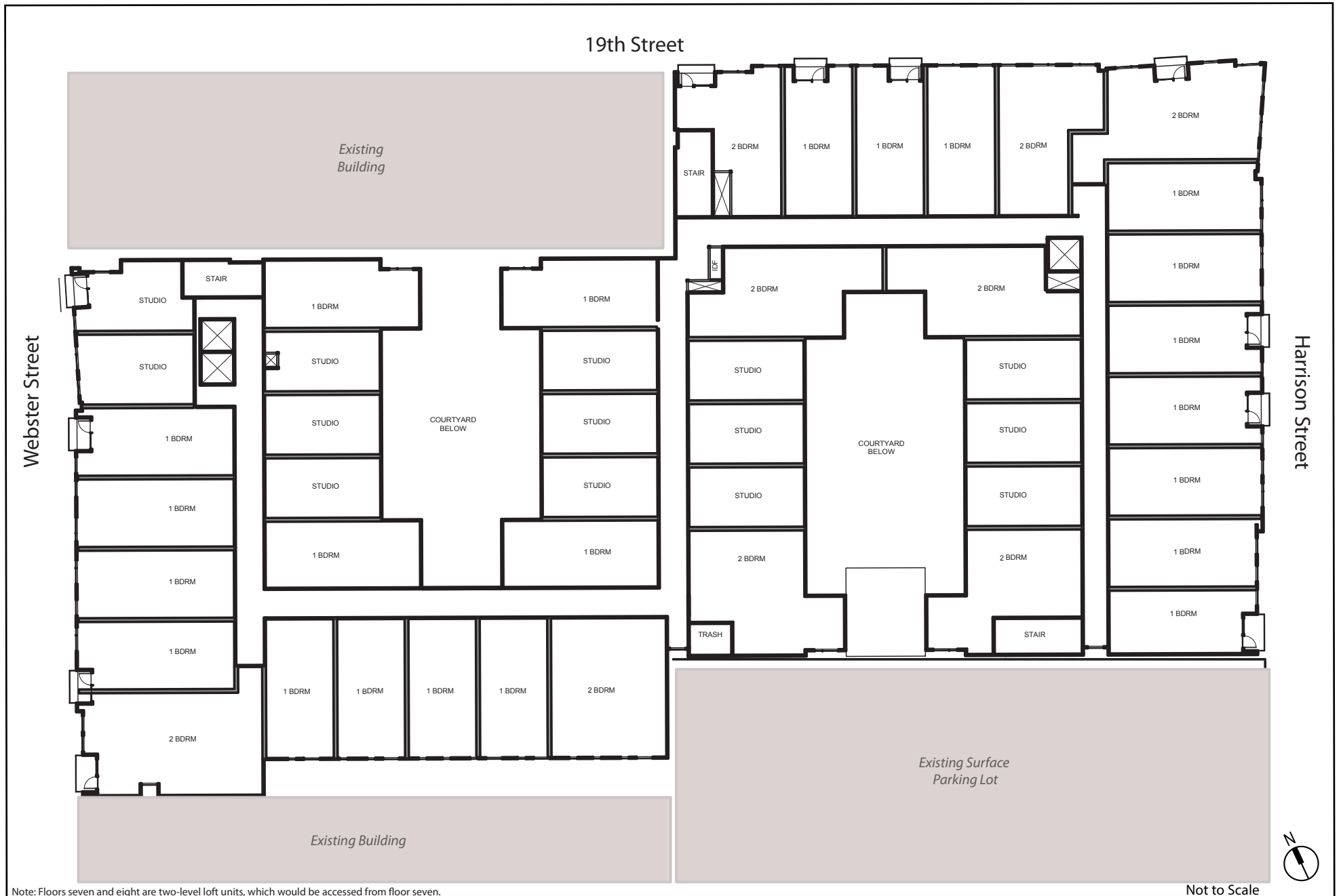
Figure 4 Typical Residential Floor Plan (Floors 4-7)
