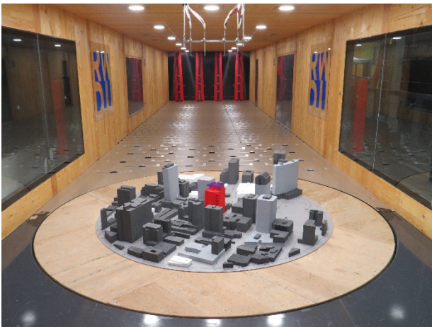
Image 2B: Wind Tunnel Study Model – Existing + Project (17-Story Tower) Configuration
