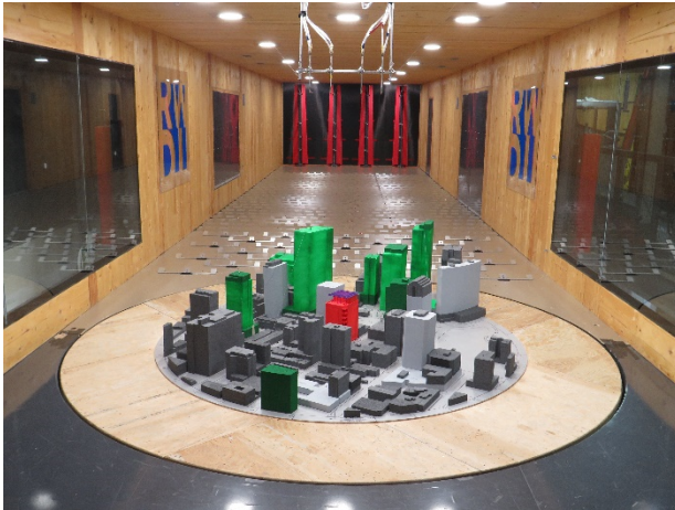
Image 2D: Wind Tunnel Study Model – Project (17-Story Tower) + Cumulative Configuration
