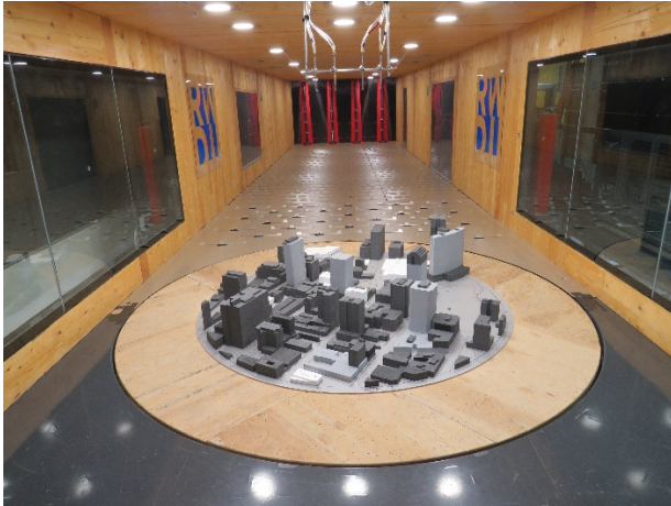
Image 2A: Wind Tunnel Study Model – Existing Configuration
