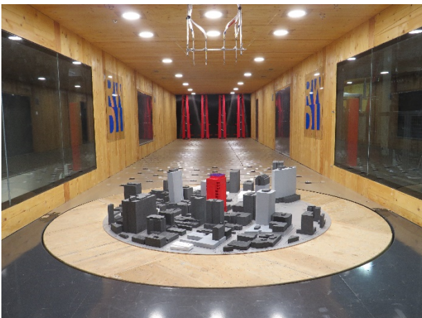
Image 2C: Wind Tunnel Study Model – Existing + Project (25-Story Tower) Configuration
