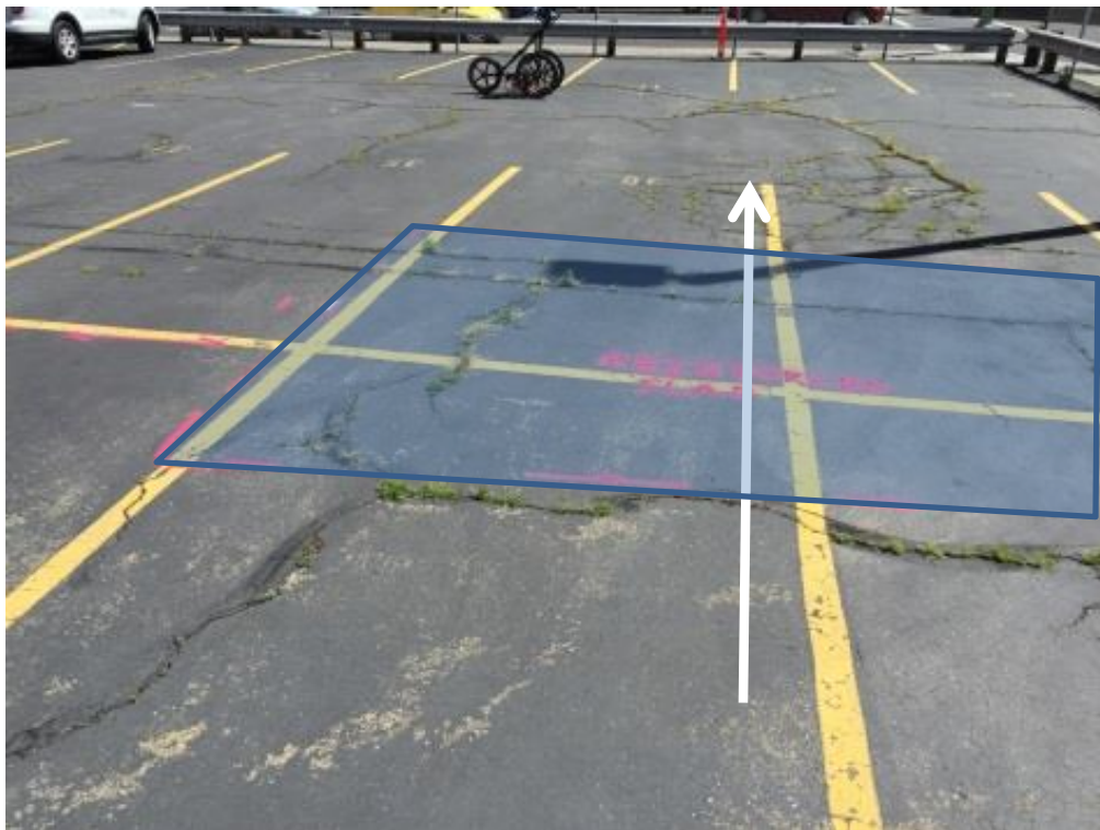
Notice area of interference in the data sample. This is the reinforced area I spoke about earlier. GPR visibility is greatly reduced due to the reinforcing
