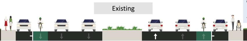
PM Peak Hour Traffic Volumes on 14<sup>th</sup> St (425 veh/hr, one way) – 2015 ~850 veh/hr is capacity for 1-lane
