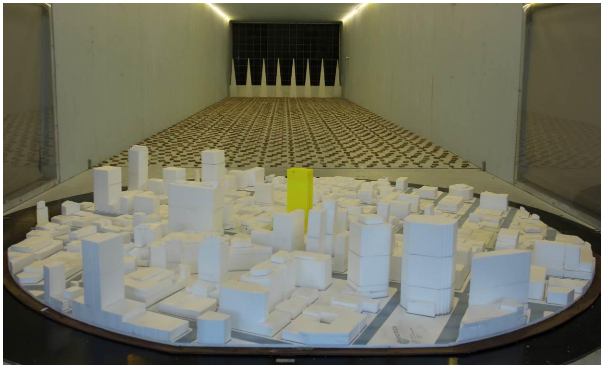
Figure 2f: Photograph of the Wind Tunnel Model (view from the west) Proposed Surrounds Scenario
