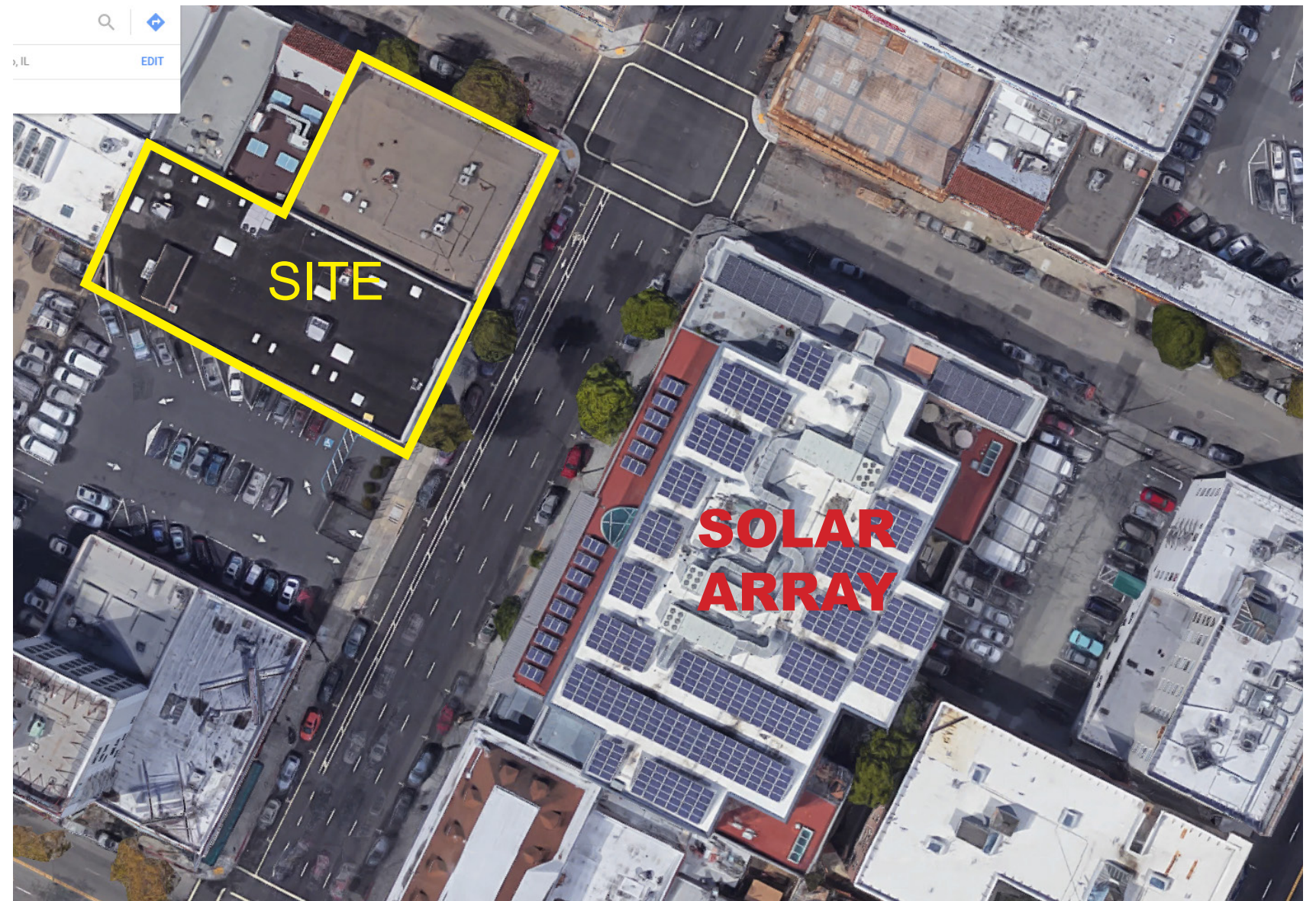
The proposed project will have an .85% reduction in yearly output of the solar array located to the projects east.
