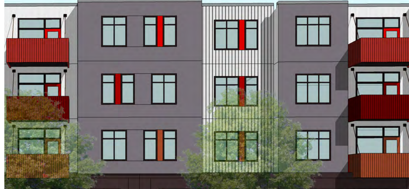
6 WINDOW @ STUCCO & CORRUGATED METAL TYP.
