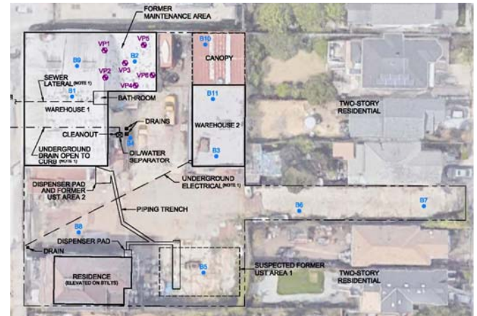
Site Plan with Historical Subsurface Investigation; RMD 2019
