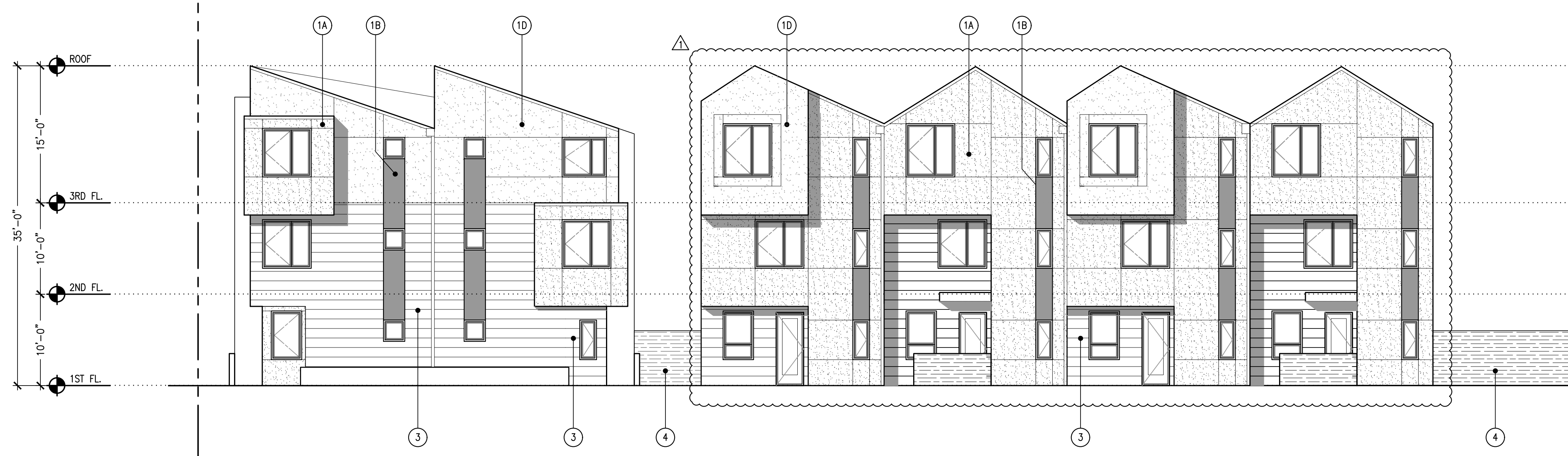
2 20TH ST ELEVATION (EAST ELEVATION) 1/8"=1'-0"
