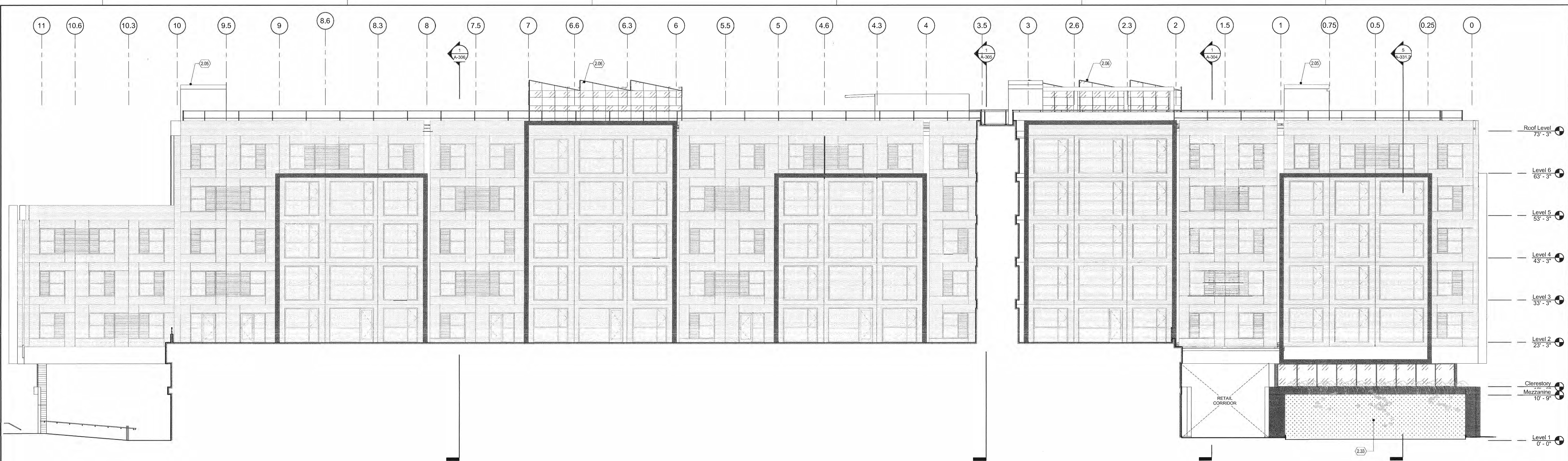
2 COURTYARD NORTH ELEVATION 1/8" = 1'-0"
