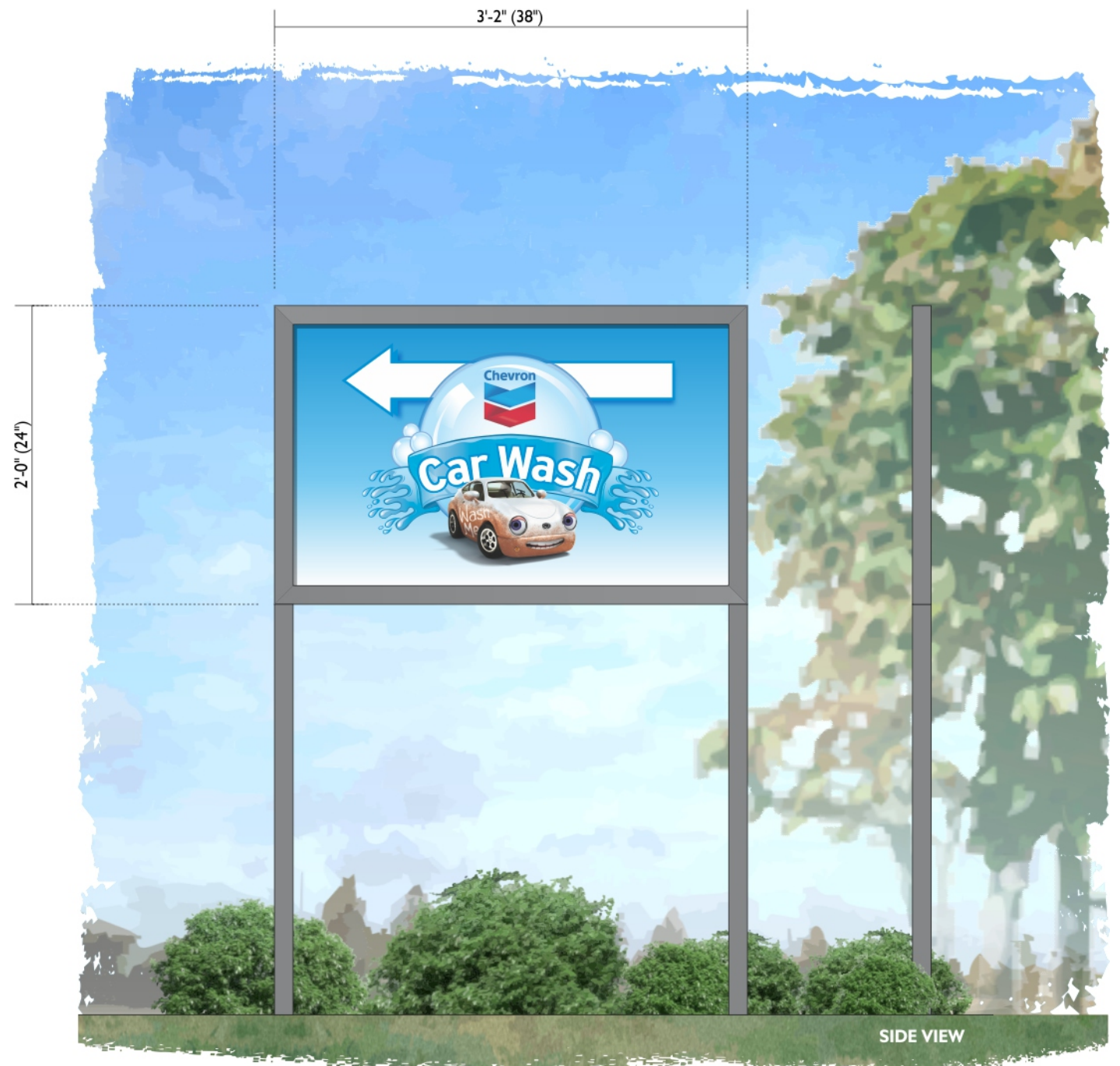
SIGN F: SINGLE FACED NON ILLUMINATED POST AND PANEL DIRECTIONAL SIGN QUANTITY: (1) / 6.3 SQUARE FEET
