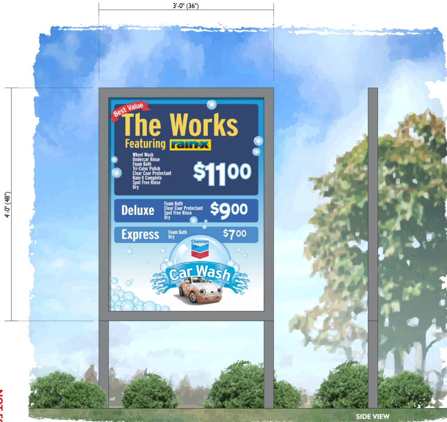
SIGN E: SINGLE FACED NON ILLUMINATED POST AND PANEL DIRECTIONAL SIGN QUANTITY: (1) / 12 SQUARE FEET
